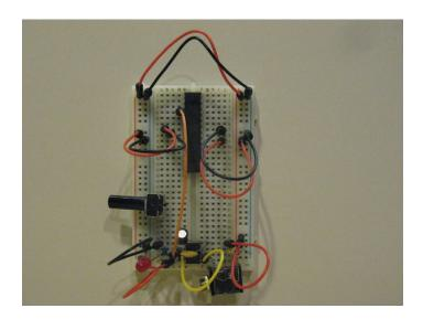
Step 22: Knob wiper to ATMEGA328 Analog Input
